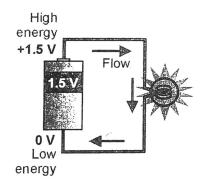
You know that water will flow from a higher tank through a hose into a lower tank. The water in the higher tank has greater potential energy than the water in the lower tank. A similar thing happens with the flow of charges in an electrical circuit.
