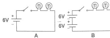
a. How much current would be measured in each circuit if each light bulb has a resistance of 6 ohms?
