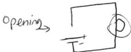
This is an open circuit. There is an opening. The lightbulb will not light up.
